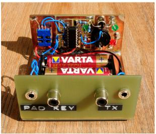
with a dremel tool as I did with my prototype shown without cover on the above pictures. This is my preferred construction method for simple circuits and I also build sturdy cabinets from solder-joined plates of this material. In this case I simply used the copperclad backside of the front plate as the circuit board.
