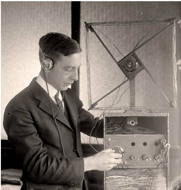
Typical early feedback audion with frame antenna
