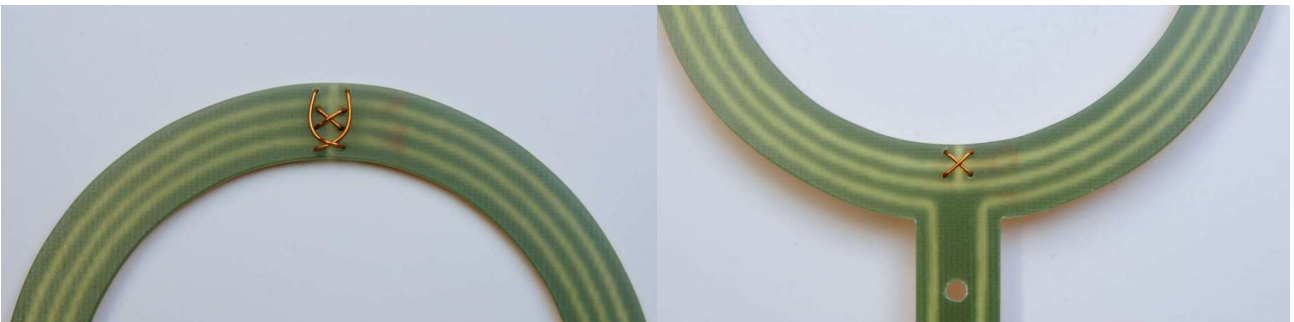
The track bridges from enameled wire were inserted through the drilled holes on the front of the loop-antenna and soldered to the copper tracks on the back.
