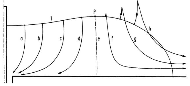
**Fig 4.** Paths of the energies which are located on field line 1 at the moment of maximum charge (**Fig 2**). Line  $e$  separates the energies which travel back to the generator during discharge from the energies which travel out into space.
