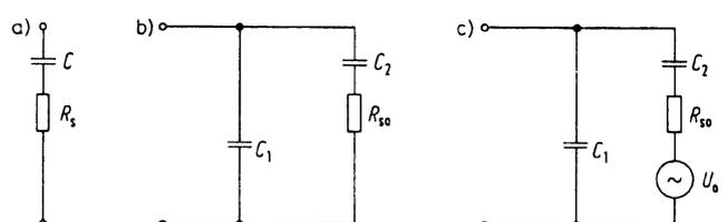
**Fig 1. Equivalent circuits for the short radiator as a transmitting (a and b) and receiving (c) antenna.**
