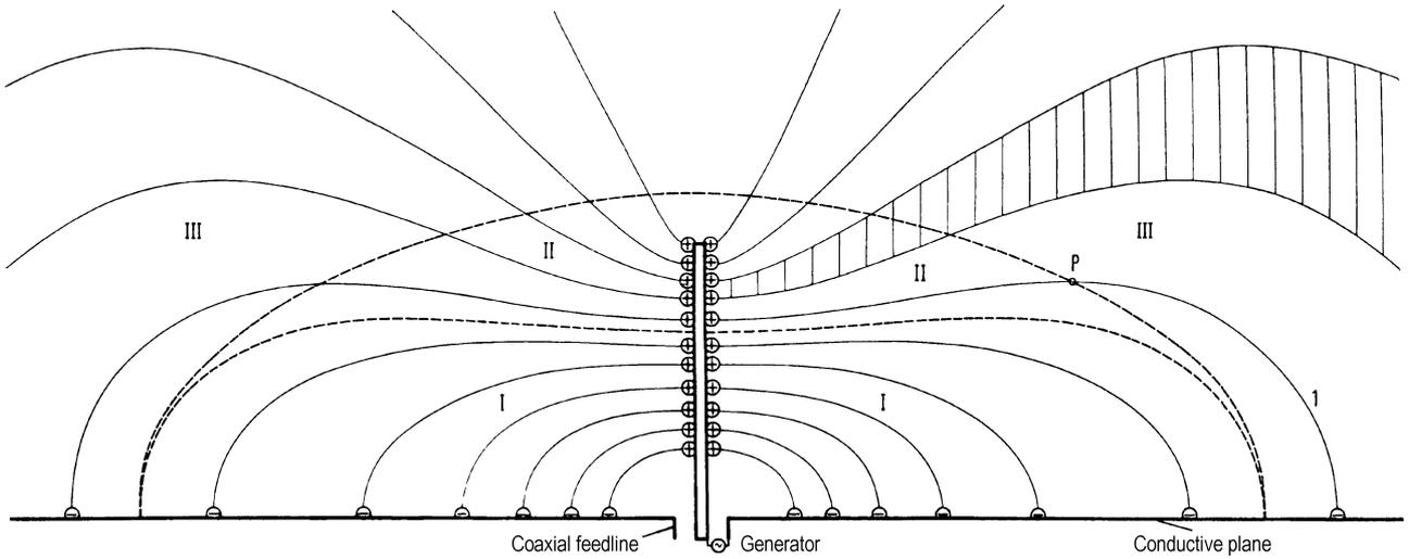
Fig 2. Electric field of a short rod antenna at the moment of maximum charge with 3 regions delimited by the broken lines; region I: dead capacitance  $C_1$ , region II: space capacitance  $C_2$ , region III: real resistance  $R_{50}$ . A section between two field lines is shown hatched.
