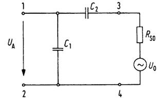
**Fig 11.** Equivalent circuit for the receiving antenna.
