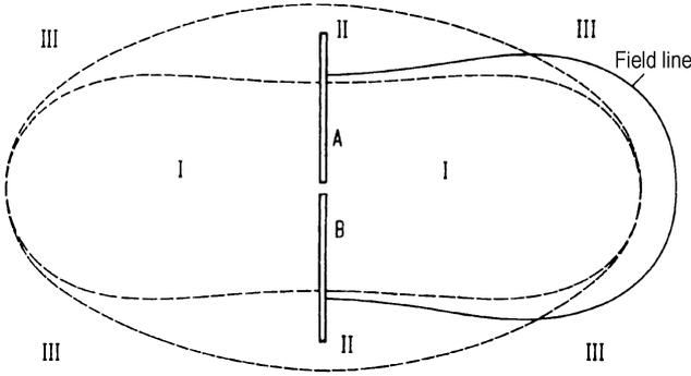
Fig 8. The three regions around a symmetrical dipole.
