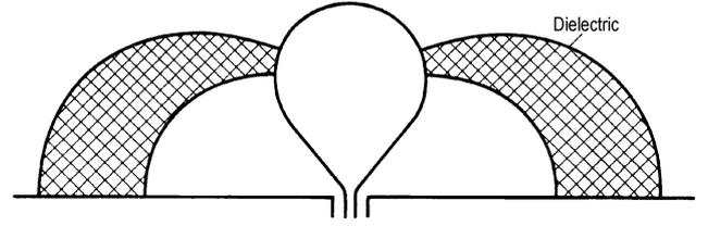
**Fig 9.** Enlargement of space capacitance by a dielectric body.
