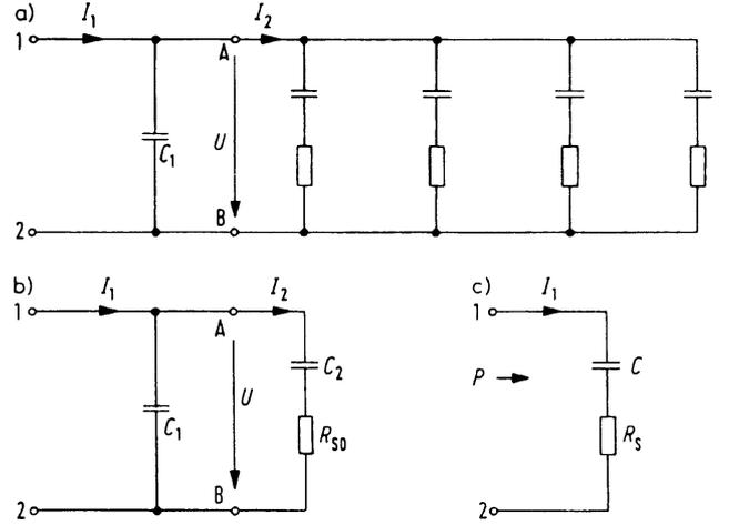
**Fig 5.** Equivalent circuits for the antenna impedance.
